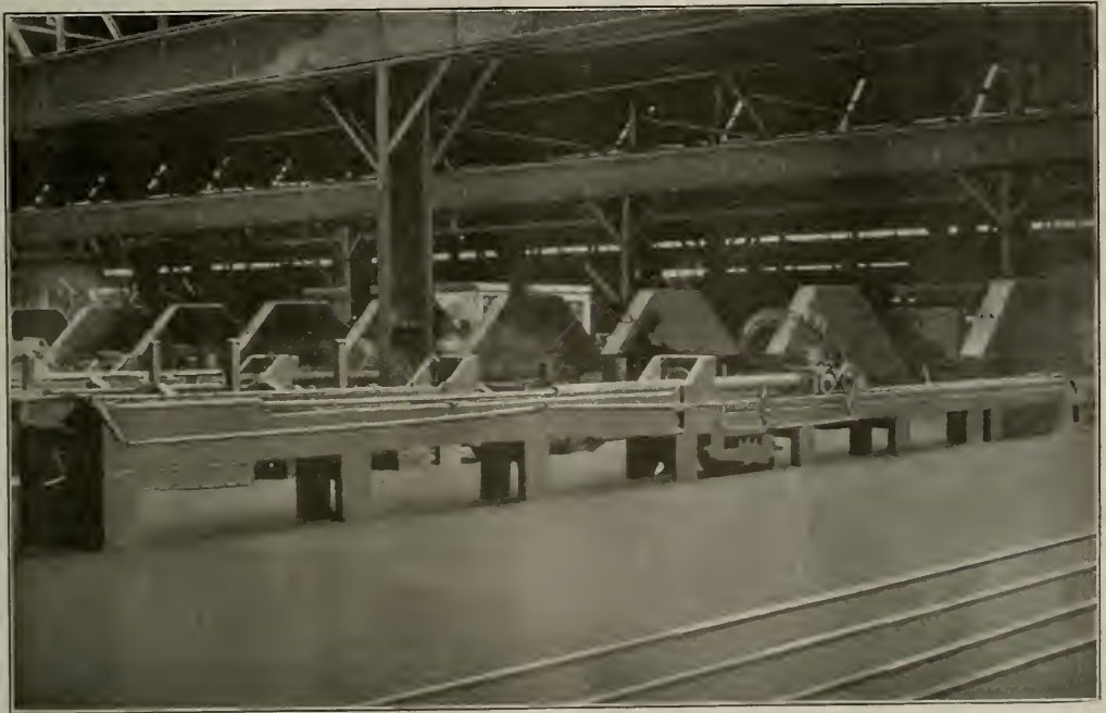
FULL LENGTH VIEW OF COLD-DRAW BENCH IN THE MANUFACTURE OF "SHELBY" SEAMLESS STEEL TUBING
